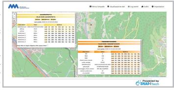
basis of traffic conditions. Snap4City, based on traffic monitoring data from some measurement points, allows the management of TAI remotely in a simple and flexible way based on the standard defined in UNI11248:2016 by sending the relevant commands for lighting regulation to the affected luminaries in multicast modality. This integrated technology offers numerous advantages for administrations and citizens, including energy savings, reduction of and emissions, and improved road safety.
