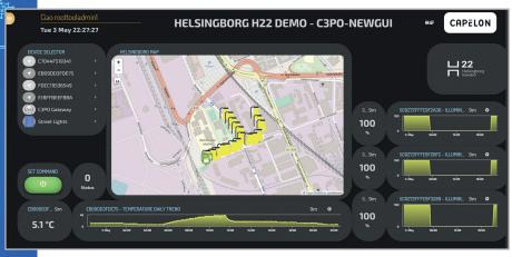
Public lighting is moving towards the usage of LED lamps and thus a strong push towards smart light solutions has been registered. They allow to be finely regulated, so that to avoid the classic on/off approach, but controlling the percentage of light needed on the basis of the actual intensity of the natural lights and contextual conditions (for
