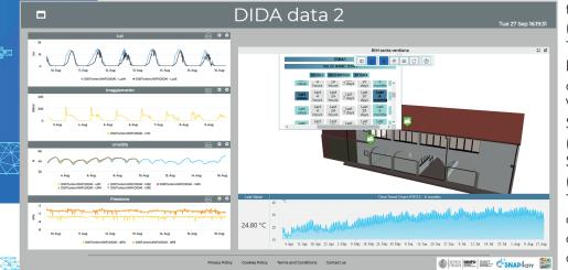
tools such as the BIM Manager (https://www.snap4city.org/730). The 3D shape is obtained by starting from formats such as IFC, DXF, SVG (Scalable Vector Graphics), STEP, IGES, STL (Stereolithography), OBJ (Wavefront), DAE (Collada), SCAD (OpenSCAD), and IV (Inventor). The Local Digital Twin also may include the detailed description of floors, detailed description of data, devices, etc.
